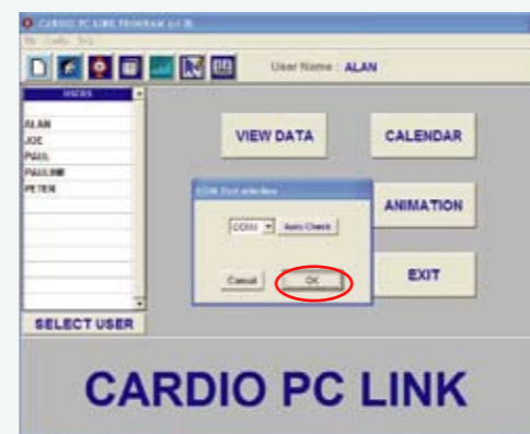
8. Then choose the COM PORT route accordingly and confirm by pressing OK.
