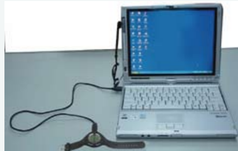
4. Plug the USB connector to the computer before opening the interface program
